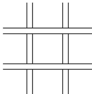
**Option D** - 3/4” round bar vertical on 6” centers through horizontal bars (3/8” x 2-1/2”) on 12” centers. All intersections are welded.
